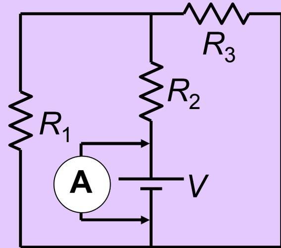
A person wishing to measure the current through the seat of EMF in the circuit above left connects an ammeter as depicted above right. Will that work?
