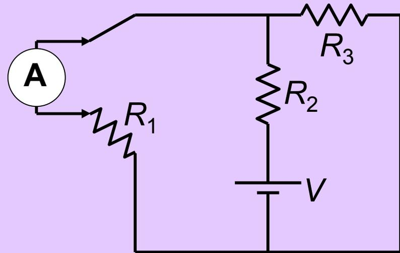
A person wishing to measure the current through  $R_1$  in the circuit above left connects an ammeter as depicted above right. Will that work?
