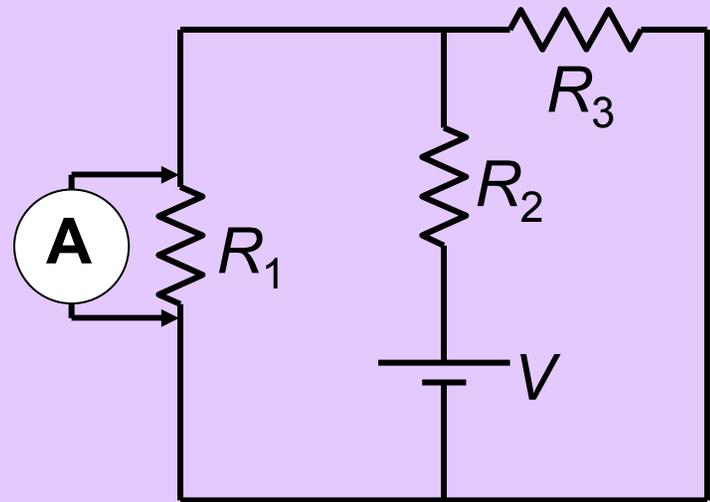
A person wishing to measure the current through  $R_1$  in the circuit above left connects an ammeter as depicted above right. Will that work?
