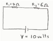
is to use the method of effective resistance. The two resistors are in series so they can be combined to form the single effective resistance  $\rm R_S.$
