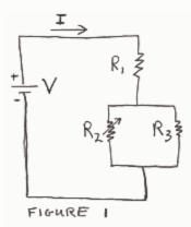
The arrow through R<sub>2</sub> in Figure 1 means that R<sub>2</sub> is a variable resistor.
