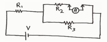
**Feedback:** An ammeter acts like a piece of wire that measures the charge flow rate through itself. To use it, in principle, one simply removes a piece of wire in that branch of the circuit through which one wishes to measure the current, and replaces that piece of wire with the ammeter.
