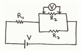
**Feedback:** An ideal voltmeter has infinite resistance. As regards the effect it has on the circuit, a voltmeter acts like dry air (unlike an ammeter which acts like a piece of wire). A voltmeter has two probes, one marked positive and the other negative. If you connect the positive probe to point A in the circuit and the other to point B in the circuit, the voltmeter shows how much higher the electric potential at A is than that at point B.
