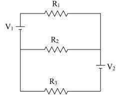
d) Clearly indicate two loops in the circuit on which one can apply Kirchoff's Loop Rule (a.k.a. Kirchoff's Voltage Law) and write the equation for each loop.
